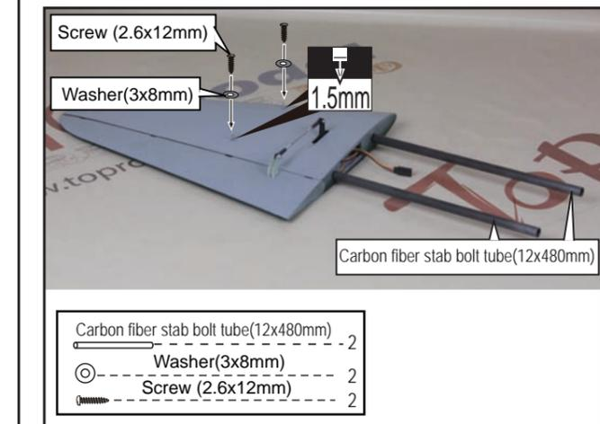
**26** Assemble the fixed stabilizer to the fuselage carefully and put the other stabilizer to the fuselage through the fiber tubes, drill holes carefully to the carbon fiber tube through the holes in the stabilizer and fix the stabilizer.
