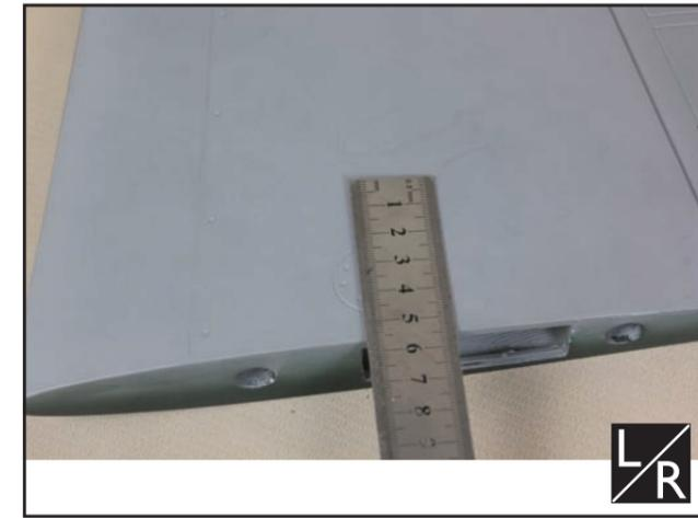
**24** Trim a slot in the stabilizer base on the mark, put the servo of elevator into the stabilizer through the hole in the wing root, install the servo to appropriate position with screws and epoxy the horn to the slot in the elevator.
