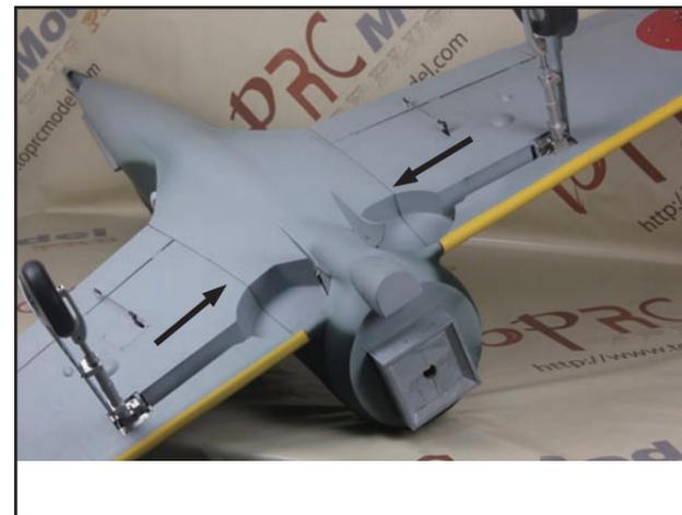
**16** Assemble the inner gear doors to the fuselage with screws and epoxy, connect the horn on the inner gear door to the servo with push rod.
