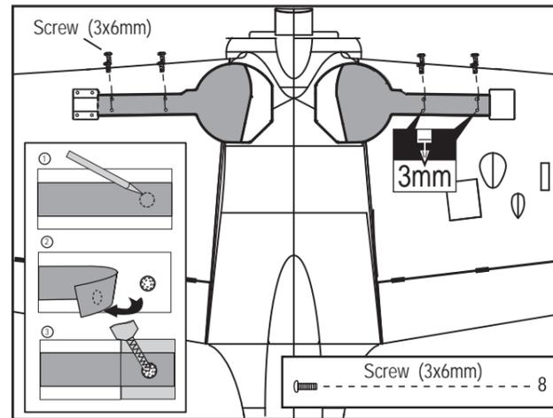
**15** Epoxy the pinned hinges, horns to the inner gear door carefully, drill holes through the gear door and pinned hinges and fix the pinned hinges tightly to the inner gear door.
