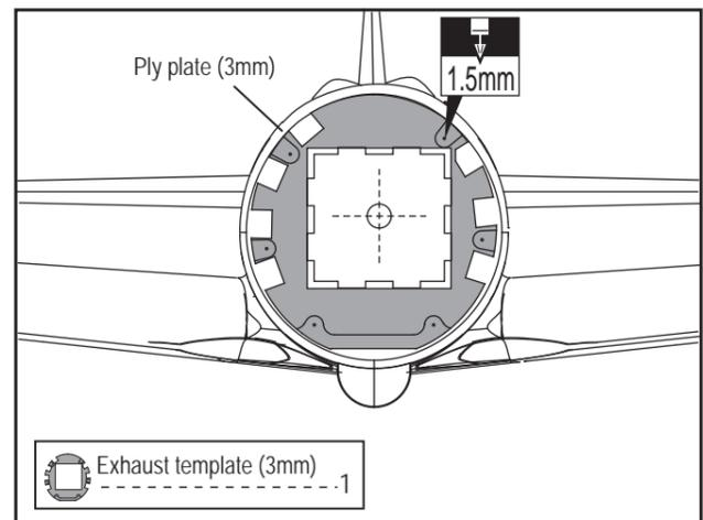
**42** Install the scale exhaust tubes and the cowling wooden frame in place on the fuselage with screws, assemble the engine to the engine mount.
