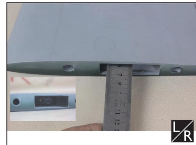
**23** Mark out the position of the elevator servo on the stabilizer.
