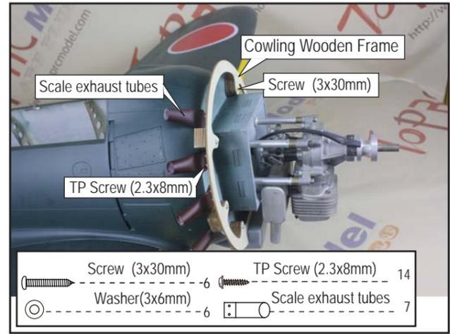
**43** Fix the cowling to the cowling wooden frame with TP screws.
