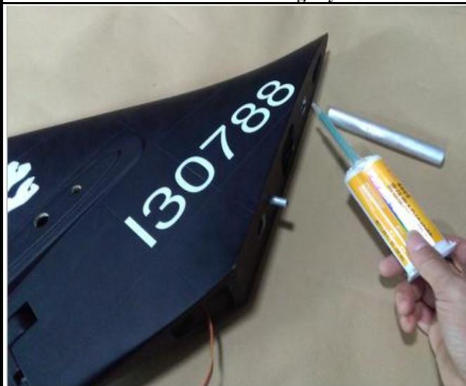
47. Offer the glue to the surface of the vertical tail section.
