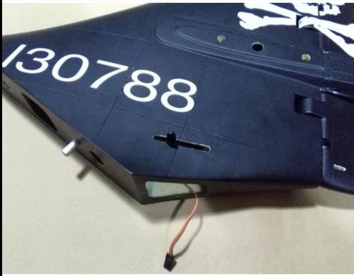
29. Trim a slot at the appropriate position in the rudder.
