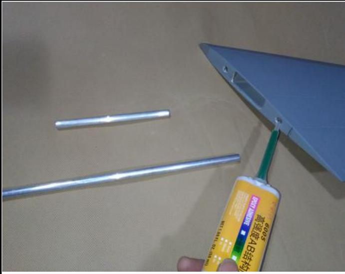
62. Fix the stab tube to the holes tightly.
