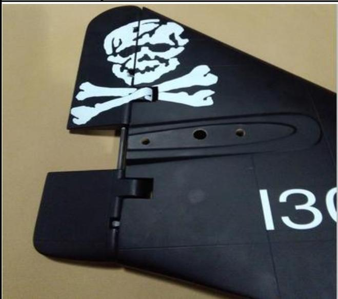
22. Apply instand type AB glue to the slots in the tail cone.
