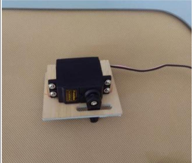
6. Assemble the servo to the wing
