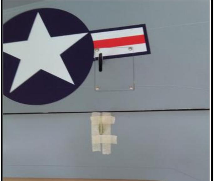
11. Connect the arm of the flap and servo arm with push rod.
