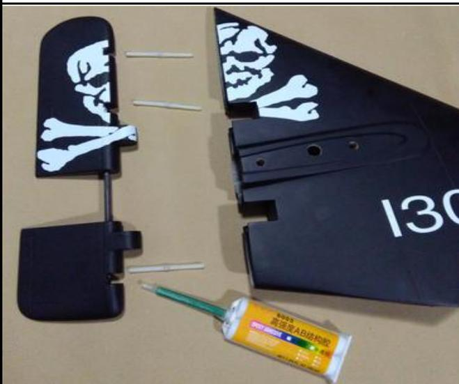
20. Apply instand type AB glue to the slots in vertical fin.
