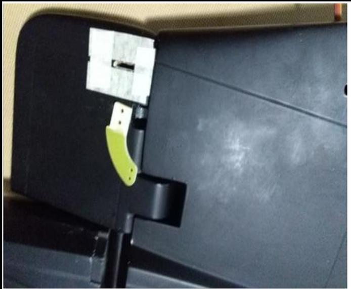
31.Glue the fiber horn to the slot tightly.
