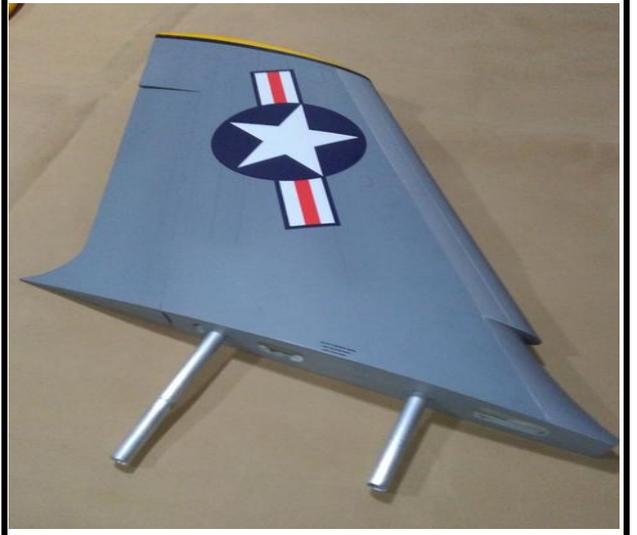
66. Assemble the wing to the fuselage and lock it to the fuselage with screws.
