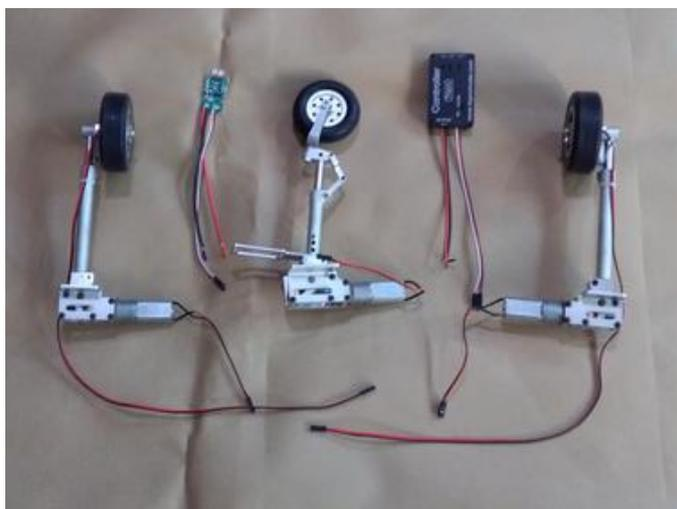
35.Assemble the retract to the fuselage with screws.
