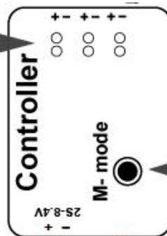
4. The M-mode button can be used for testing the e-retracts without remote control nor receiver.
