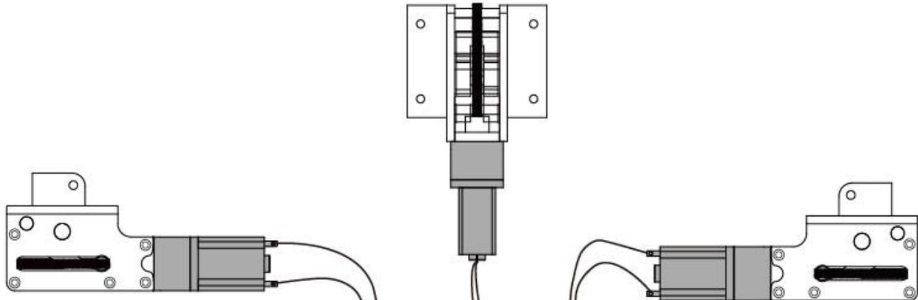
2. Turn on the radio control to check the lights on the circuit board, if the lights turn on green or turn on red orderly 0.5 second after each from the right to the left and all the lights will turn off after 15 seconds, then the circuit will work normally. Otherwise the circuit will be a defective one if you make sure the setting on your radio control are correct, please don't use it but contact with your supplier in time.
