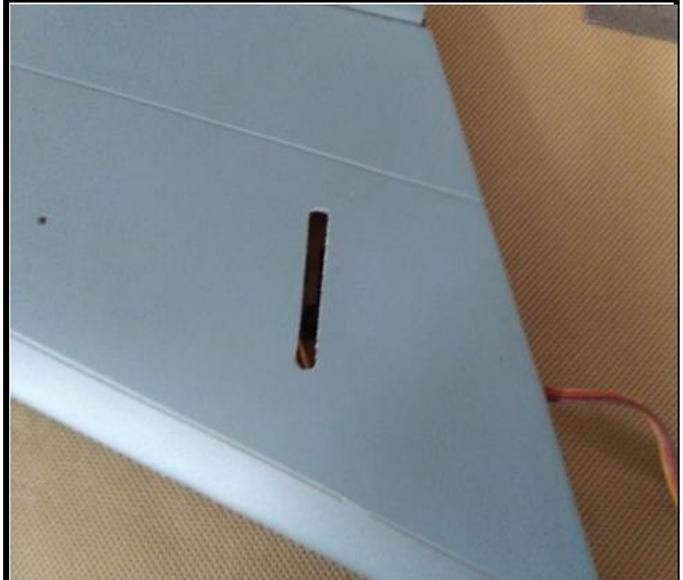
17. Glue the horn to the elevator and assemble the servo to the stabilizer.
