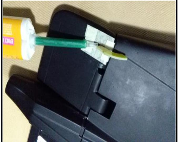
32.Remove the masking tape after the glue dried.
