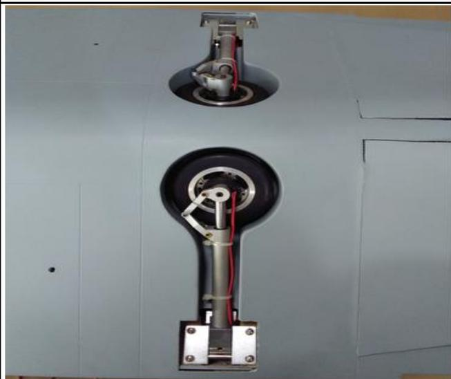
37.The sketch map of the nose gear and nose gear servo parts.
