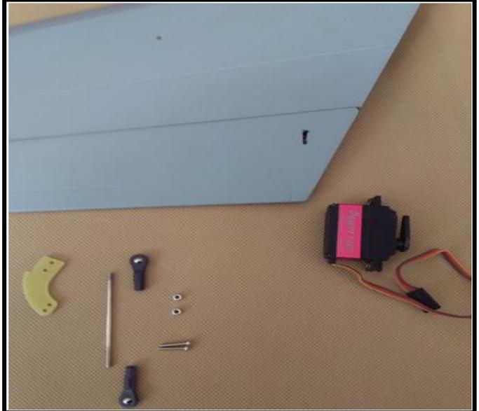
15. Measure the depth and mark out where the servo would location.
