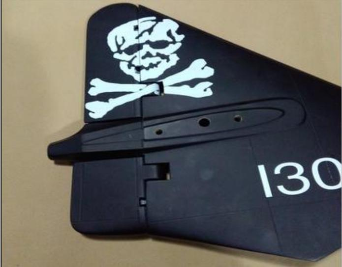
24. Measure the depth of the rudder servo position.
