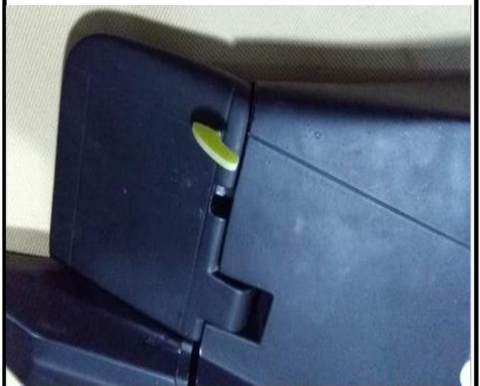
33.Connect the servo arm to the rudder fiber horn .
