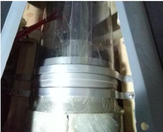
57. Mark out the position in the air intake and fuselage where there need to be hollowed.
