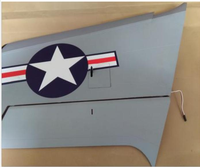
7. Drag the servo line out of the wing.
