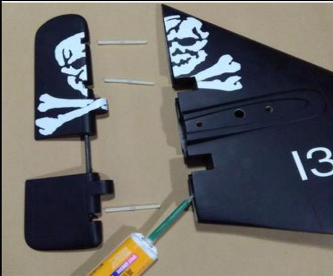
21. Assemble the rudder to the vertical fin and make sure it can move freely.
