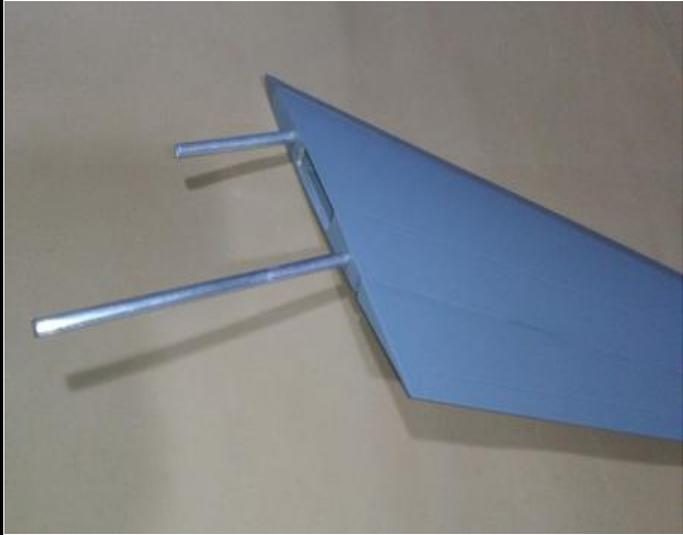
63. Assemble the stab to the fuselage and lock it to the fuselage with screws.
