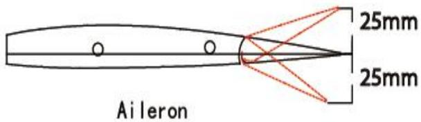
69. Adjust the travel of each control surface to the values in the diagrams. These values fit general flight capabilities. Readjust according to your needs and flight level.
