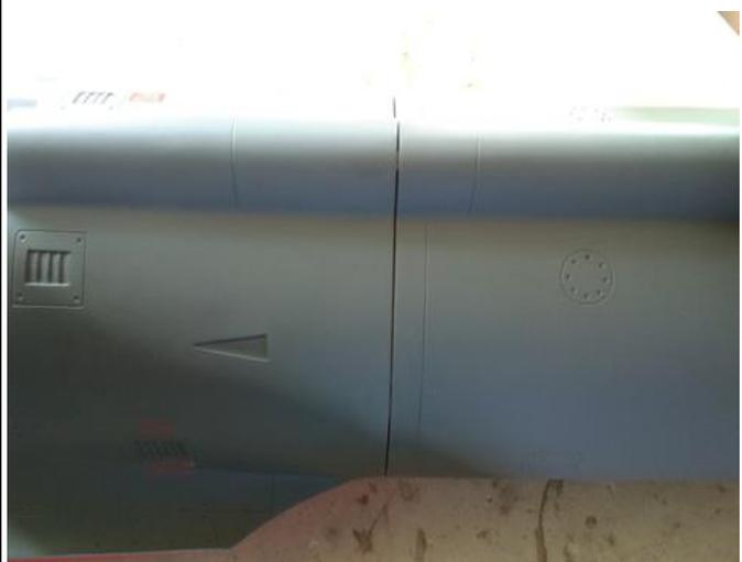
38.Assemble the fuel tank to the fuselage.
