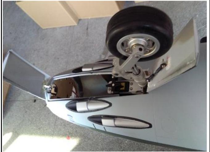
30. Connect the back half nose gear door to the landing gear with push rod and screws.
