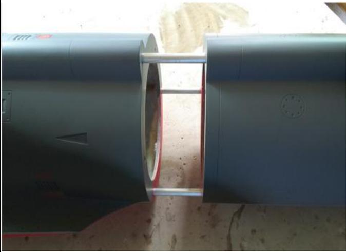
37.When the fuselages be assembled together, fasten them with screws from the fuselage.
