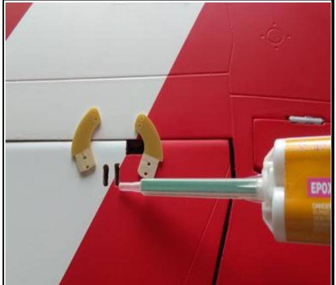
**5. Apply AB glue to the slots in the flaps and assemble the horns into them.**
