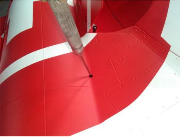
42.Assemble the stab to the fuselage through the stab tubes and lock them with screws.
