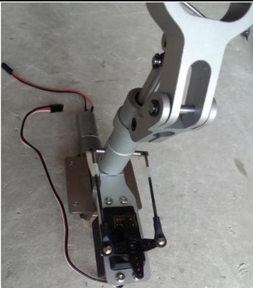
29. Assemble the nose retract to the fuselage with screws and assemble the back half nose gear door.
