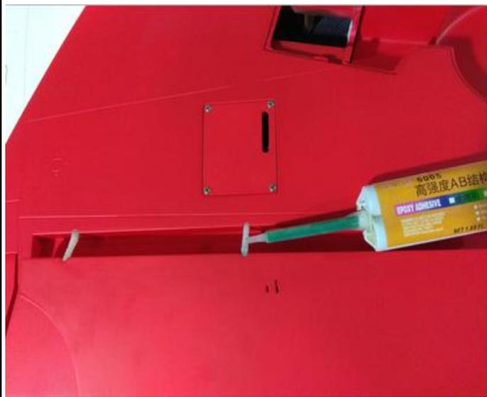
**2. Epoxy the flap to the wing, Keep some space about 1mm width between the trailing edge and the flap.**
