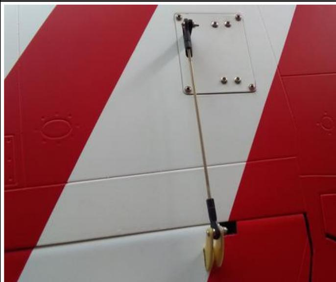
9. Fix the servo trays with servo assembled to the wings with screws.
