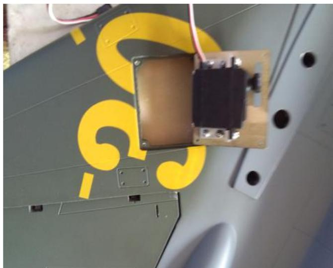
18. Connect the fiber horns to the servo arms with the linkage and lock each side with screws and locknuts.
