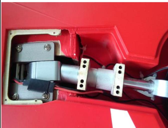
34.Assemble the main gear door to the landing gear with screws.
