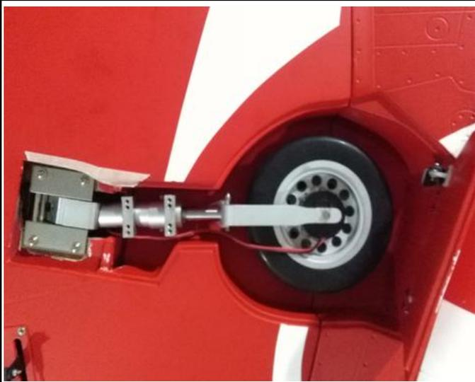
33.Glue the plies to the socket rings on the landing gear.
