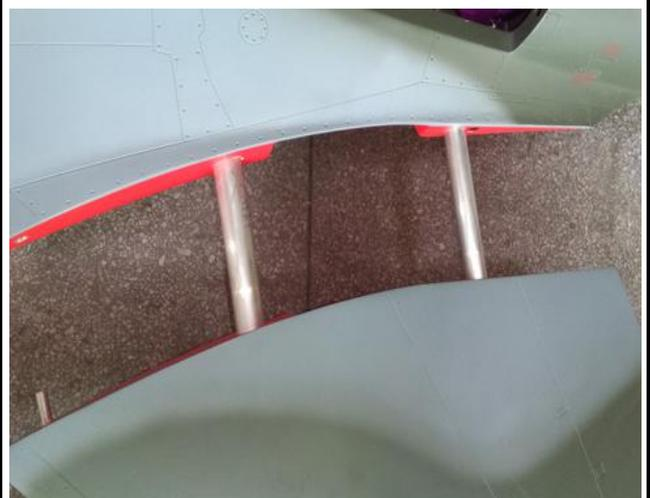
41.Lock the wings from the holes on the bottom fuselage with screws.
