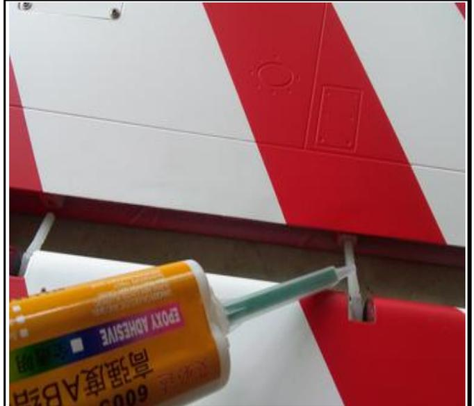
**4. Apply AB glue to the slots in the ailerons, and assemble the horns into them.**
