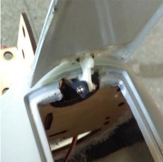
28. Assemble the nose landing gear and the servo to the nose retract.
