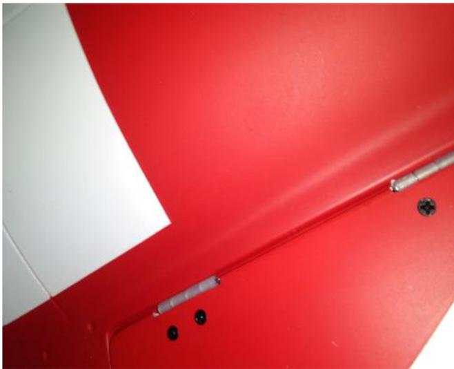
22. Assemble the inner gear door to the fuselage with screws and epoxy.
