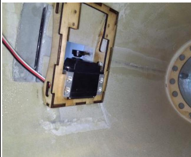
20. Connect the plastic horn in the belly brake to the servo arm with the linkage and lock each side with screws and locknuts.
