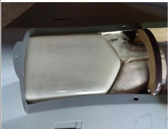
39.Assemble the engine and tail pipe to the fuselage with screws.
