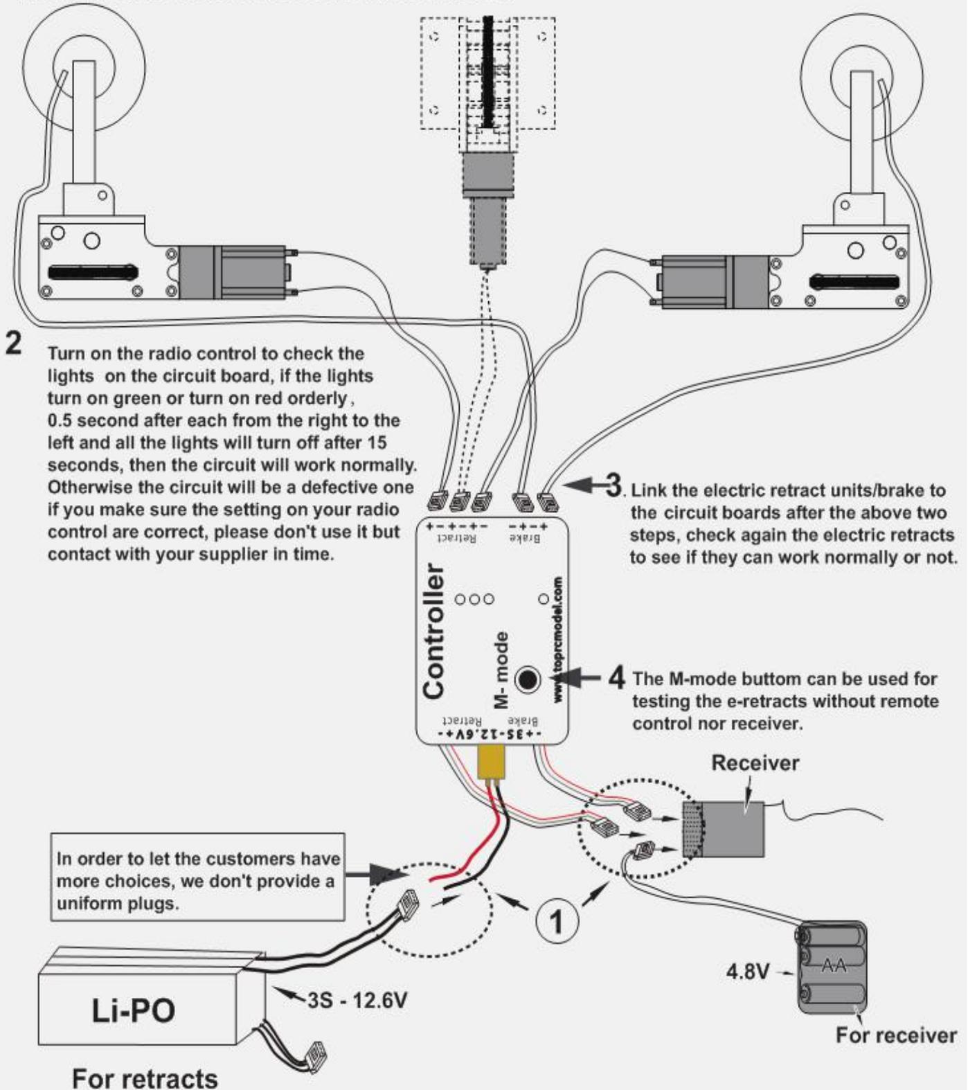
Assemble the electric retracts to the plane after several times smoothly running.
