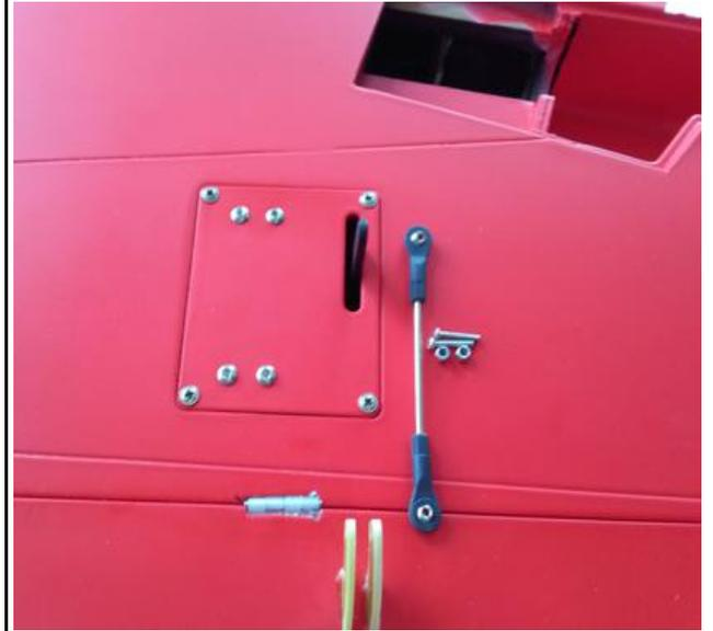
10. Connect the fiber horns to the servo arms with the linkage and lock each side with screws and nut.
