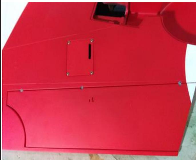
**3. Apply instand type AB glue to the holes in the aileron and hinges. Epoxy the aileron to the wing.**
