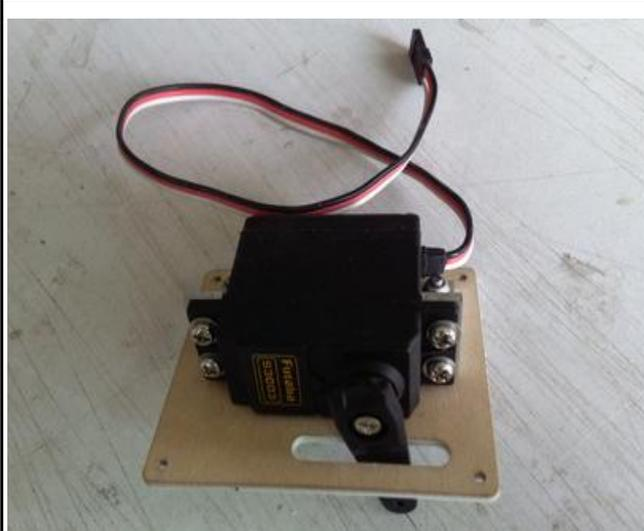
15. Assemble the servos to the stab servo trays.
