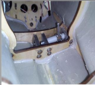
44. Connect the pushrod to the arm on the stabilizer joiner.
