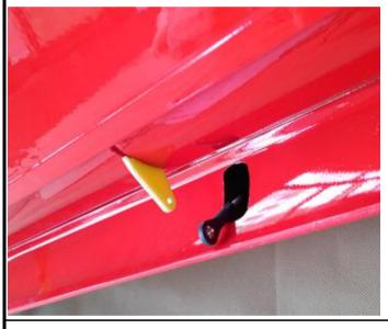
14. Assemble the linkage to the horns with screws.
