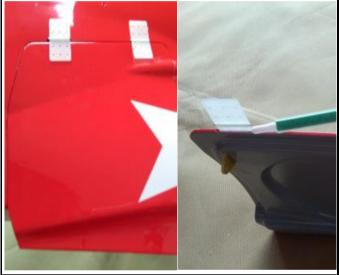
**32.** Cut surplus the pinned hinges, put the wheel doors to the fuselage via the opened slots.
