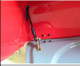
40. Connect the linkage to the fiber horn with screws and locknuts.
