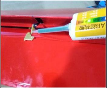
15. The sketch map when the horns in the wings assembled finished.
