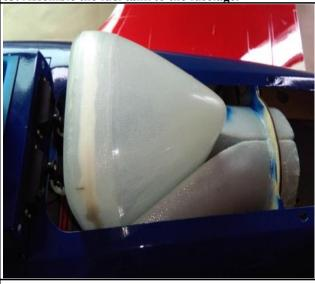
64. Assemble the fuselage hatch.
