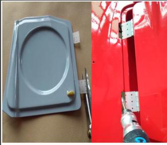
33. Drill holes to appropriate position in the fuselage and lock the wheel doors with screws.
