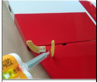
21. Assemble the servo to the vertical fin.
