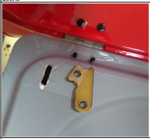
38. Epoxy the fiber horns to the wheel doors.
