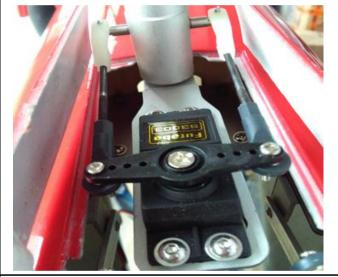
51. Put the retract to the appropriate position from inner fuselage.
