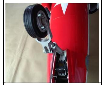
53. Connect the hatch hinge to the clevis on the Alu sash with screw.
