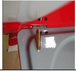
**39.** Connect the linkage to the fiber horn with screws and locknuts.
