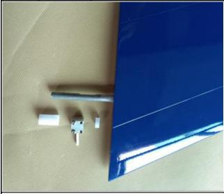
43. Assemble the stabilizers to the fuselage.
